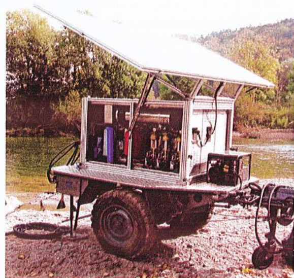
Trunz Water Trailer - a mobile solar powered water treatment plant for disaster relief & military application
