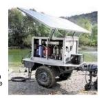
The Trunz Water Trailer purifies water in two stages: an automatic back flushing prefiltration system removes larger particles. In a second stage, a reverse osmosis system removes contamination such as viruses, bacteria and dissolved solids.
