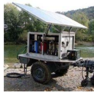
The Trunz Water Trailer with solar power
